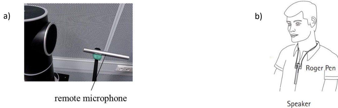
Fig. 10. a) WRMS placement of the Roger Pen (Hussetdt et al., 2021) and b) usual placement of the Roger Pen (Phonak, no date b)
