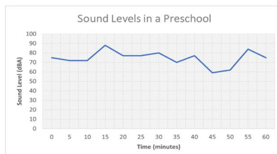
Fig. 3. Sound levels measured every 5 minutes in a preschool at the child's ear level over the course of an hour.
